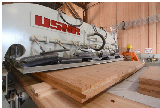
Figure 5 USNR CLT Pneumatic press for 3, 5, and 7 (max 10.5" thickness) panels (<10' wide, max length 24'. Photo credit, DR Johnson, OregonCLT.com.
