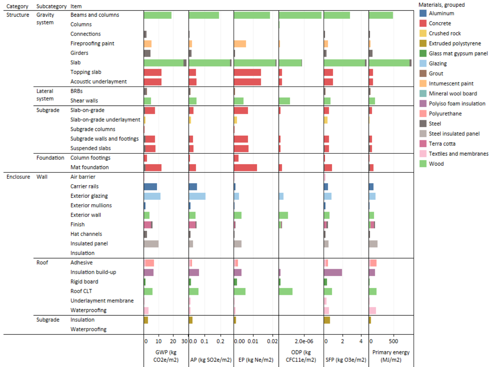
Figure 16. All impact categories by building category, subcategory, and item, life cycle stage A.
