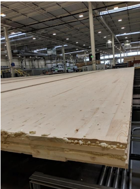
Figure 7. CLT panel after layup, glue application, and pressing
