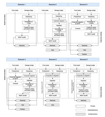
Fig. 2 System boundary of the treatment scenarios for treating 350 tpd of sewage sludge generated from the proposed cavern STWs and 105 tpd of food waste in Hong Kong
