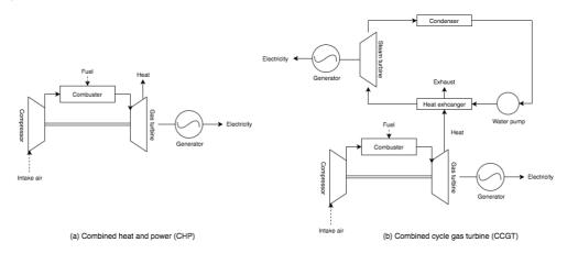
Fig. 1 Schematic diagrams of (a) CHP system and (b) CCGT system
