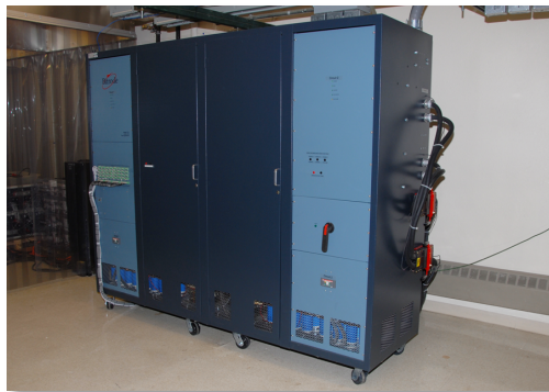
72 V 1000 A Bitrode (2 Channels)
