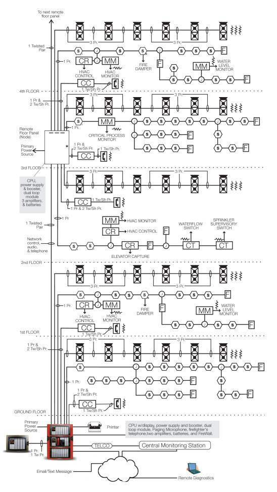
System design benefits greatly from this huge capacity. Minimal cabling requirements take scalability a step further. With EST4 a single copper pair or single fiber supports panel network data, audio data, as well as telephone data. This cuts cable counts by up to 75 per cent. Meanwhile, multiple firefighter's telephones risers are accommodated on the network, which allows them to be deployed at much further distances compared with analog audio transmission methods.
