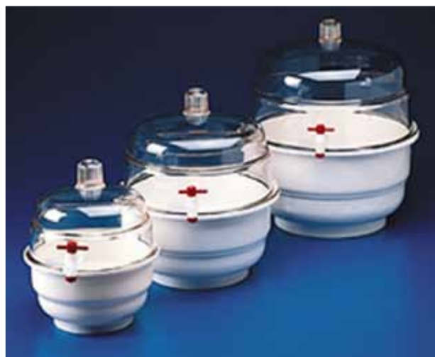
140, 190 and 230 mm plate capacity (Vacuum Models Shown)
