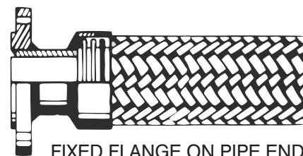
FIXED FLANGE ON PIPE END
