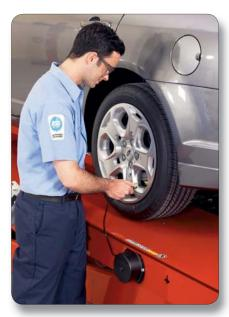
Integrated inflation hoses, located at each wheel position, retract when not in use to keep the work area clear.
