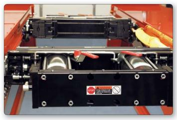
Swing air jacks flip up when not in use to provide maximum clearance.
