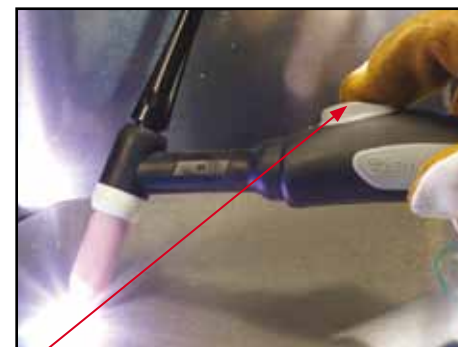
(5) Press the torch switch and the arc will ignite across the gap between the tungsten and work piece. Hold even distance of about 2mm gap between the tungsten and work piece to maintain the arc.
