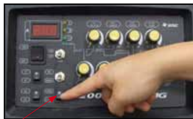
(6) Set the Pulse Selector switch to Pulse
