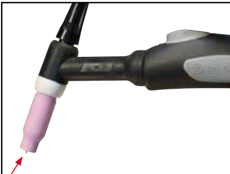
(9) Assemble the front end torch parts using the correct size and type of tungsten electrode for the job, the tungsten electrode does not require a sharpened point for AC welding
