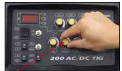
(4) Set the Pulse Frequency at 2 Hz
