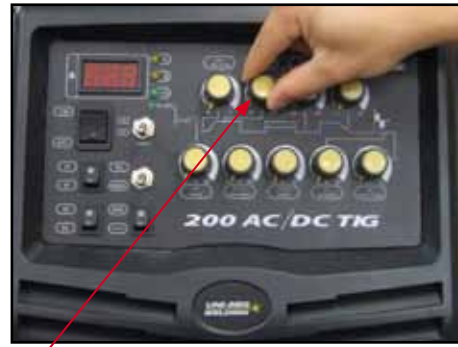
(3) Set the Peak Current (amps) to suit the tungsten size material type and thickness to be welded.
