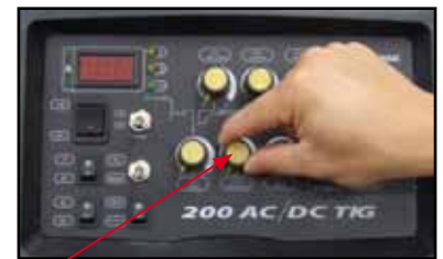
(4) Set the Pulse Frequency at 2 Hz
