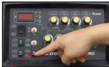
(6) Set the Pulse Selector switch to Pulse
