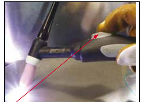
(14) Press the torch switch and the arc will ignite across the gap between the tungsten and work piece. Hold even distance of about 2mm gap between the tungsten and work piece to maintain the arc.
