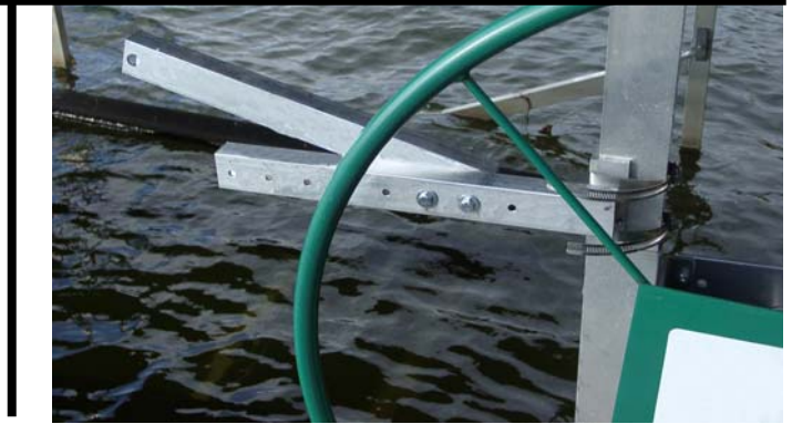
FIG 11: Right Winch Post Installation View
