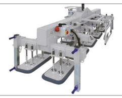
Special VacuMaster Vario with lift capacity of 10 t (special applications with lift capacity over 2 t on request)
