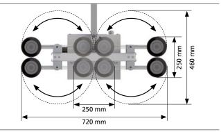
Vacuum gripper spacing with adjustable suction feet (VacuMaster Light 100-4)
