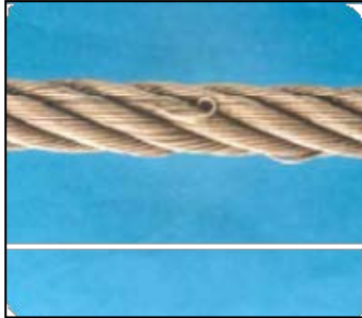
Damaged steel wire rope
