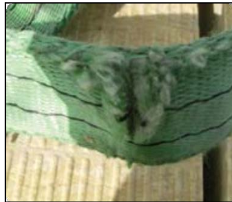
Sling damaged on sharp edges
