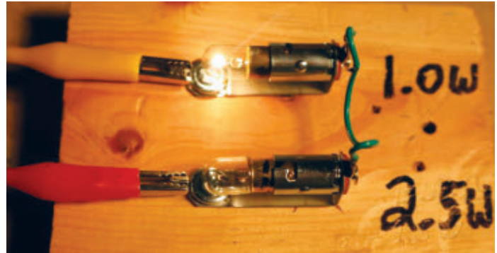
FIGURE 10. When driven in series, the bulb with the higher watt rating glows very dimly.
