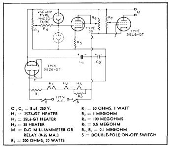
Fig. 5—Fast-acting circuit for relay or measurement operations.
