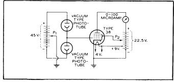
Fig. 7—Sensitive circuit for matching measurements.
