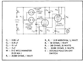
Fig. 10—Circuit for measurement of light-intensity ratios.
