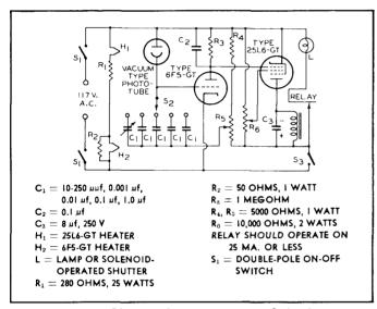
Fig. 12-Photographic-exposure control circuit.
