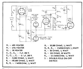
Fig. 9-A-C operated sensitive circuit for matching measurements.
