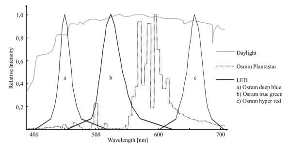
Fig. 1. Relative spectral distribution of radiation of the used light sources (edited; Nilsen, 1971; Osram, 2009; Osram, 2010; Osram, 2011)
