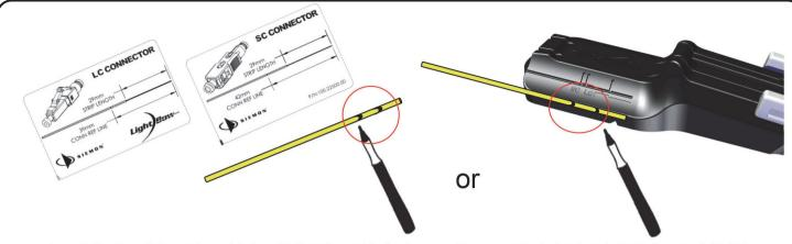
Locate the template card provided and follow the guide for the specific connector being terminated. The card depicts proper strip lengths for both SC and LC connectors. With the end of the fiber placed even with the end point shown on the template card, mark the strip length as shown. Also place the additional reference line mark indicated to be used as a visual aid during the insertion step.
