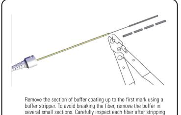
to verify the buffer coating is also removed. Sometimes mistaken
