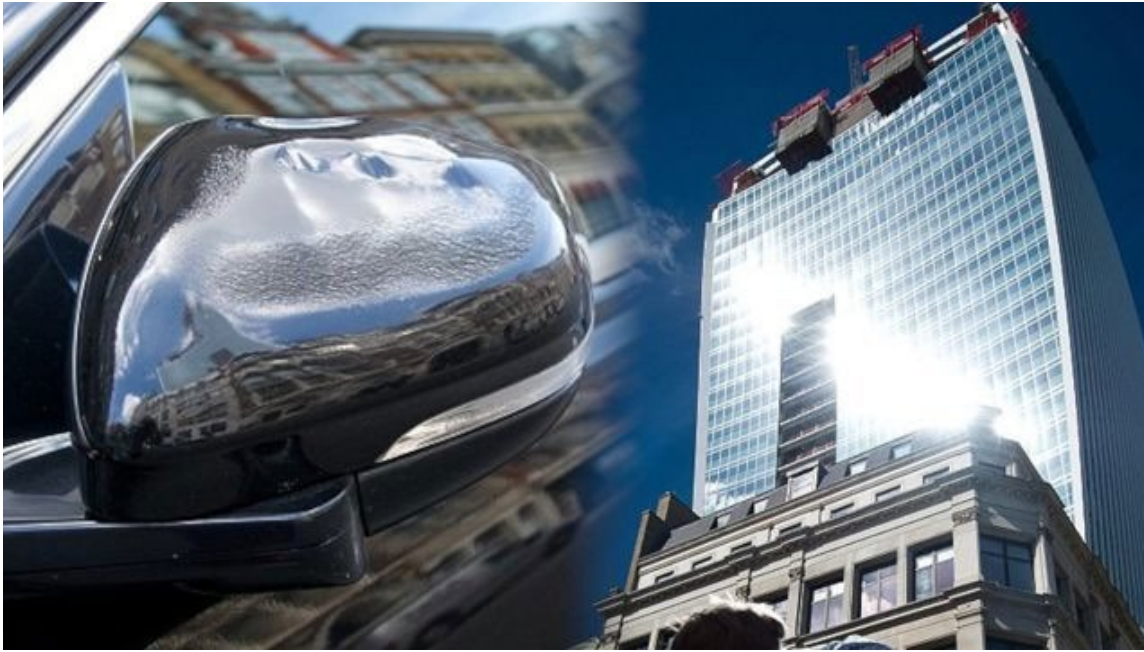
FIGURE 17 External obstructions can redirect sunlight through reflection, reaching areas that otherwise would be in the shadow. The photograph shows the heat effects of reflected sunlight being concentrated through reflection off a high reflectance curved façade. The concentrated reflected sunlight deformed a car mirror.
