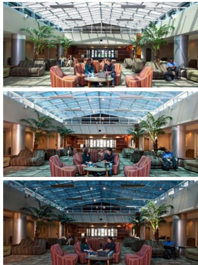
FIGURE 46 Photographs of atrium with electrochromic glazing at high (top), medium (middle), and low (bottom) transmittance states.
