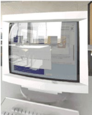
FIGURE 3 Glare from veiling reflections off a computer monitor, that compete with the brightness of the screen, producing visual discomfort.
