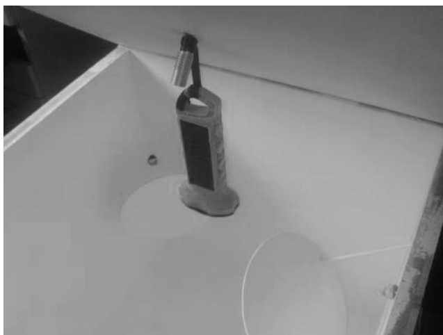
Figure L.1 – Interior view of photometer box with suspended light
