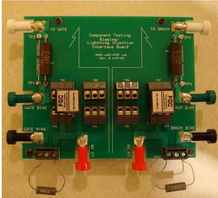
**Figure 5:** Component Testing Biasing/Lightning Injection Interface Board.
