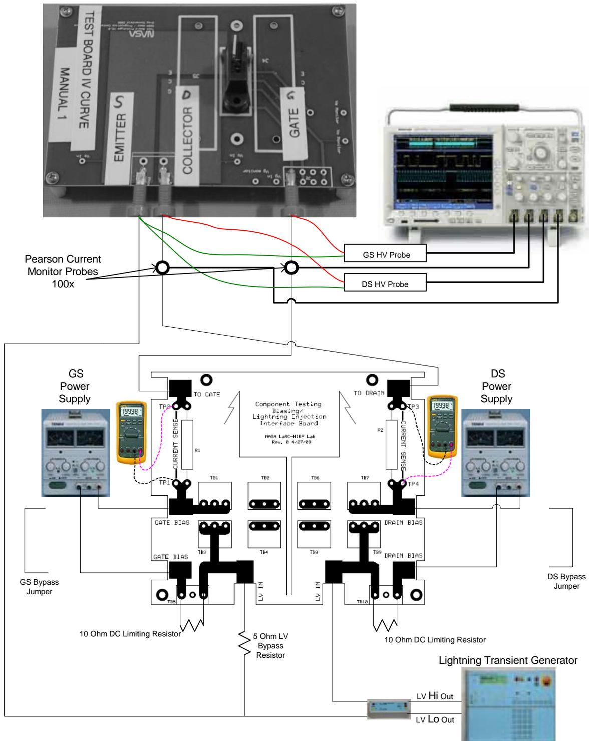
**Figure 6:** Pin Injection Test Hookup diagram. (HV Lines were each  $81.5''+43.0''=124.5$  inches long. Two sections allowed connection-to/bypass-of Attenuator Box.)
