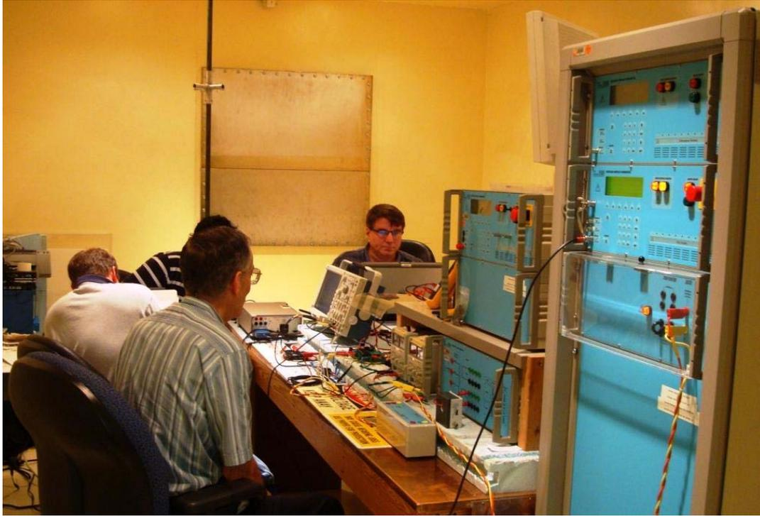
**Figure 3:** Lightning-generating equipment was used for pin-injection tests. (EMC Partner MIG0600MS shown on right.)
