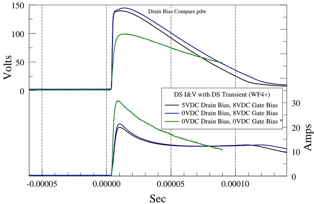
**Figure 11:** Drain ON versus Drain OFF Comparison. Peak Voc= 240V WF4+ was injected into the DS terminals, with  $V_{GS-bias}$ = 8VDC and  $V_{DS-bias}$ = 5VDC (Black) versus 0VDC (Blue, Bypassed). (Device AO, Tests 19 & 20.) \*Data are also shown from NASA/TM-2009-215794 testing (Green), where 240V WF4+ was injected across DS terminals with no other circuitry connected to the MOSFET. (Device H1, Test 214)
