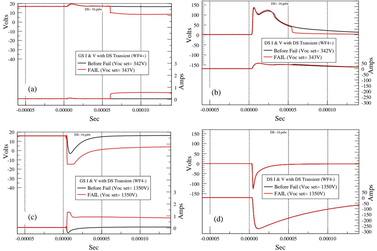
**Figure 16:** Comparison of Fail Levels with WF4+ and WF4- injected into MOSFET DS terminals. (WF4+,  $\odot$  D-S pin config. Top: a & b.) (WF4-,  $\ominus$  D-S pin config. Bottom: c & d.)  $V_{GS-bias} = 16$  Volts for these data. The plots on the right (b & d) are the DS voltages and currents. The plots on the left (a & c) are the corresponding GS voltages and currents resulting from the injection on the DS terminals.
