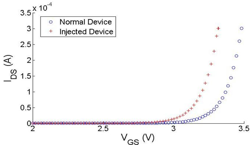
**Figure 25:** Turn-On characterization for lightning injected device in GS configuration, injection intensity M, strokes = 10 and gate bias = 8V.
