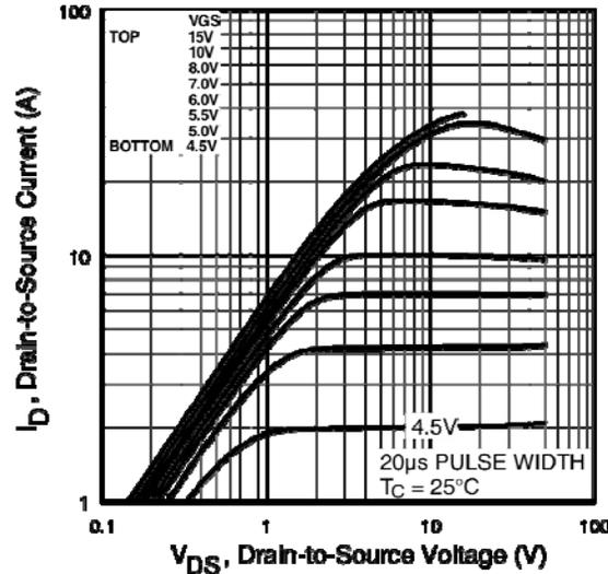
Figure 10: I-V Curves for IRF520PBF (25 Deg. C).
