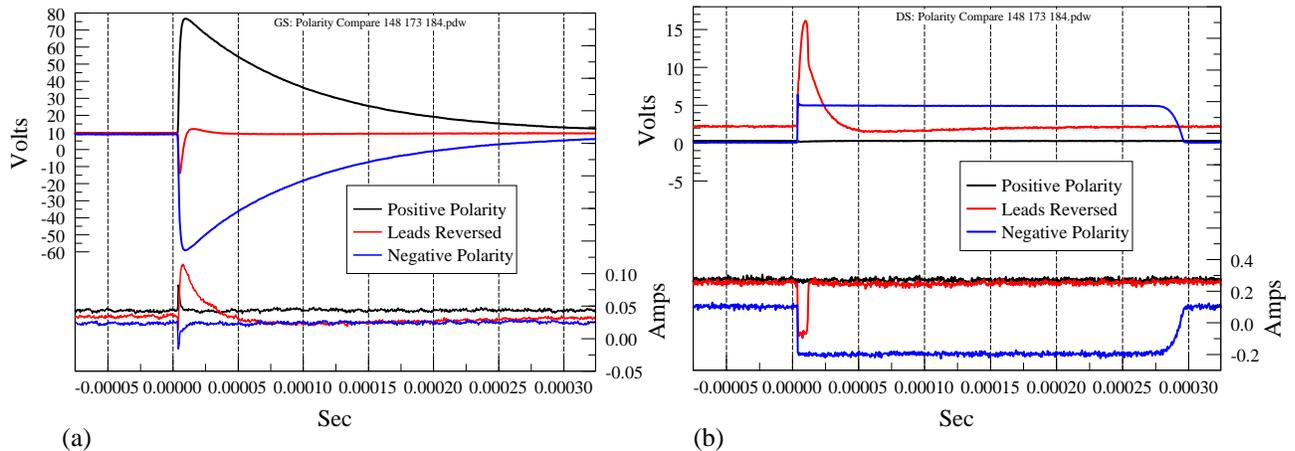
**Figure 12:** Comparison of Positive Polarity, Lead Reversal and Negative Polarity. Peak  $V_{oc} = 70V$  WF4 was injected into the G-S terminals, with  $V_{GS-bias} = 8VDC$  and  $V_{DS-bias} = 5VDC$ . (a) Shows the GS voltages and currents. (b) Shows the D-S voltages and currents.
