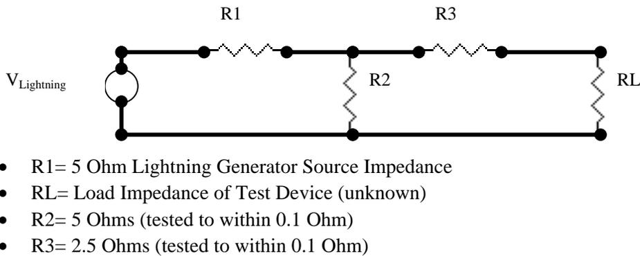
**Figure 8:** Circuit Schematic to enable Waveform 4 testing down to 40V Peak with MIG0600MS Transient Generator.
