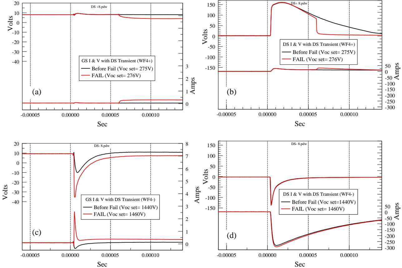
**Figure 14:** Comparison of Fail Levels with WF4+ and WF4- injected into MOSFET DS terminals. (WF4+, ③D-S pin config. Top: a & b.) (WF4-, ③ D-S pin config. Bottom: c & d.)  $V_{GS-bias} = 8$  Volts for these data. The plots on the right (b & d) are the DS voltages and currents. The plots on the left (a & c) are the corresponding GS voltages and currents resulting from the injection on the DS terminals.
