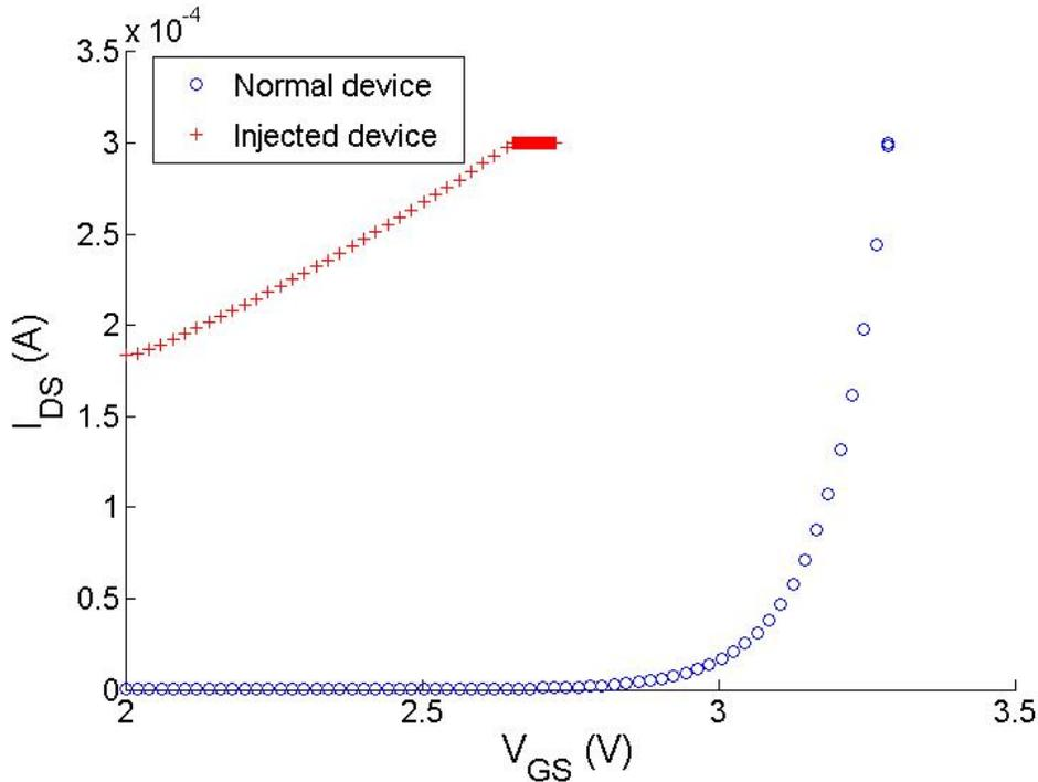
**Figure 22:** Turn-On characterization for lightning injected device in GS configuration, injection intensity H, strokes = 20 and gate bias = 8V
