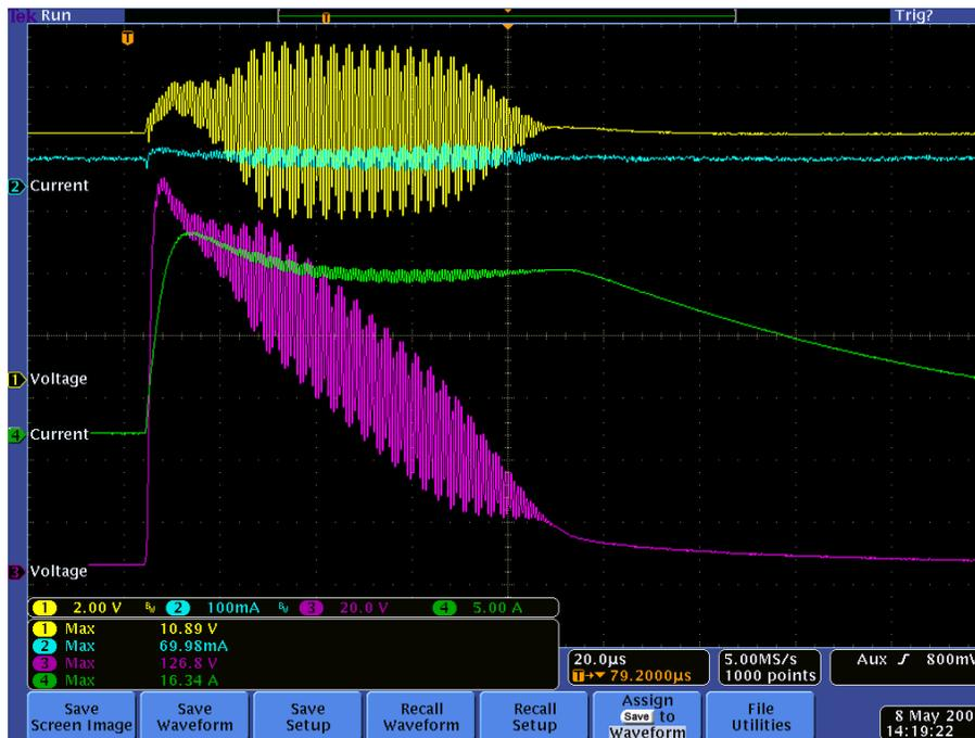
**Figure 19:** Oscilloscope display of “ringing” phenomena. (Ch. 1:  $V_{GS}$ , Ch. 2:  $I_{GS}$ , Ch. 3:  $V_{DS}$ , Ch. 4:  $I_{DS}$ )
