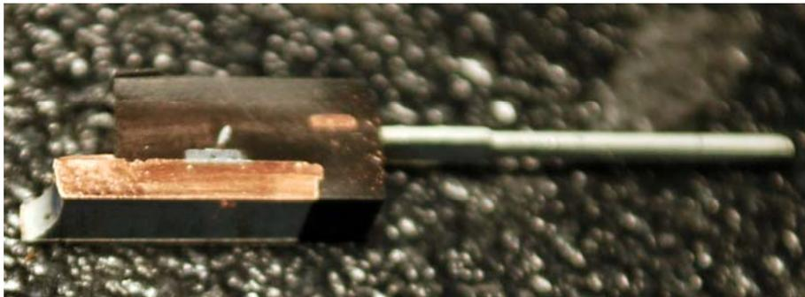
**Figure 21:** Cross Section cut performed on IRF520 MOSFET.
