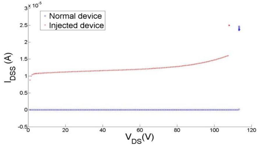
**Figure 23:** Leakage characterization for lightning injected device in GS configuration, injection intensity H, strokes = 20 and gate bias = 8V.
