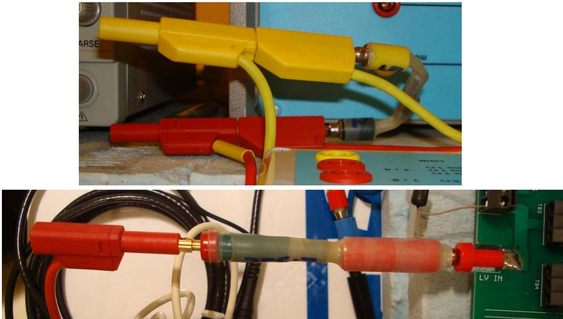
**Figure 9:**  $R2 = 5 \text{ Ohms}$  (in parallel, top photograph),  $R3 = 2.5 \text{ Ohms}$  (in series, bottom photograph), implementation.
