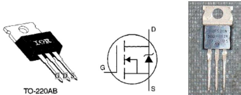
**Figure 1:** IRF520NPBF MOSFET package (left), Schematic (center) and photograph (right). Gate, Drain and Source are labeled “G”, “D”, and “S”, respectively.
