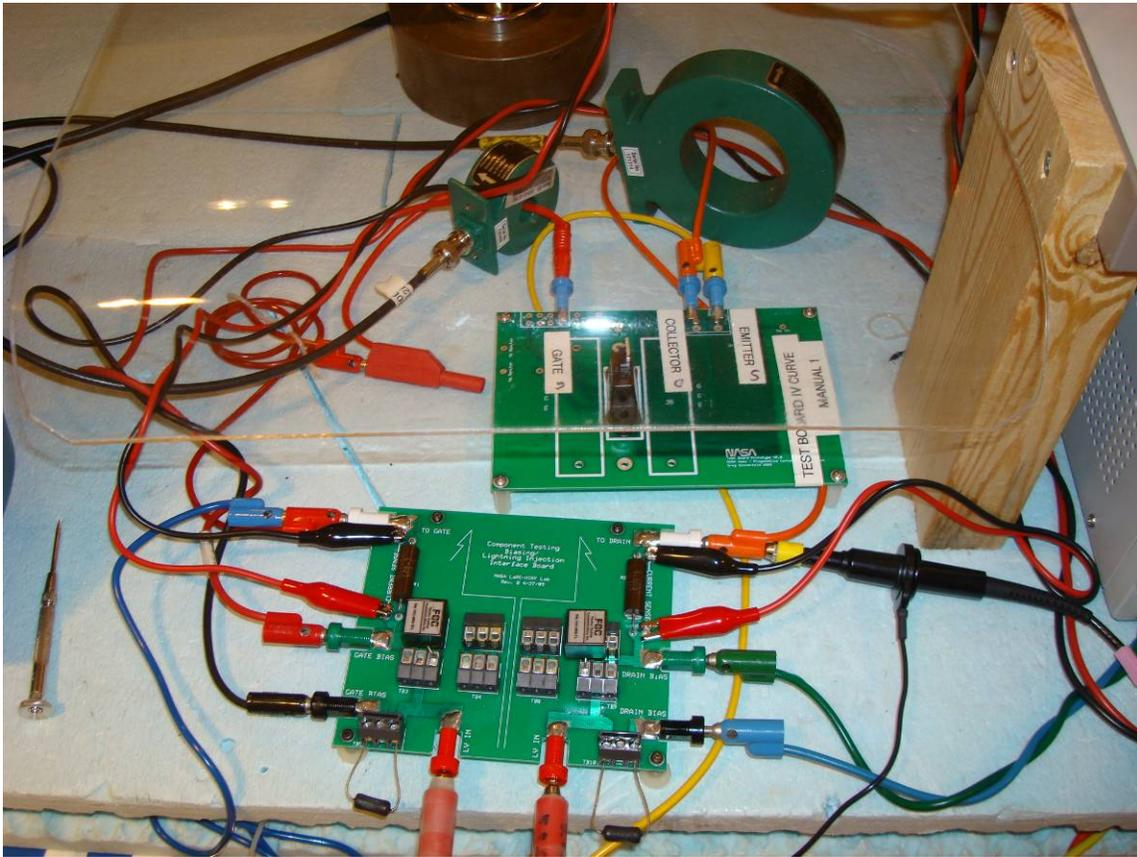
**Figure 7:** Pin Injection Test Hookup Photograph
