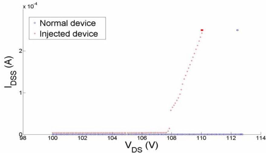
**Figure 24:** Breakdown characterization for lightning injected device in GS configuration, injection intensity H, strokes = 20 and gate bias = 8V.
