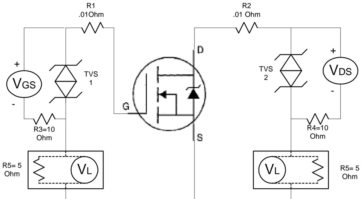
**Figure 4:** Pin Injection Test Setup Schematic.
