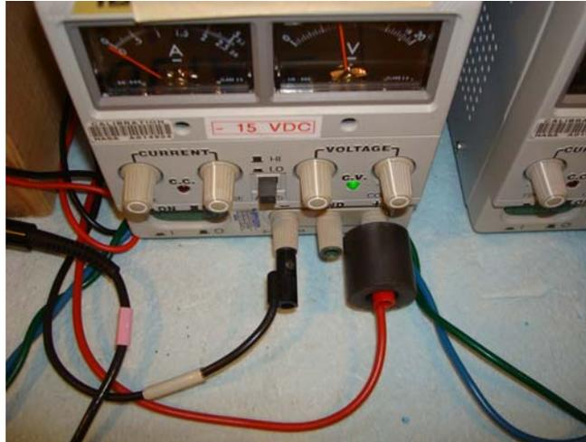
**Figure 20:** Installation of ferrite core on  $V_{GS+}$  Power supply terminal.
