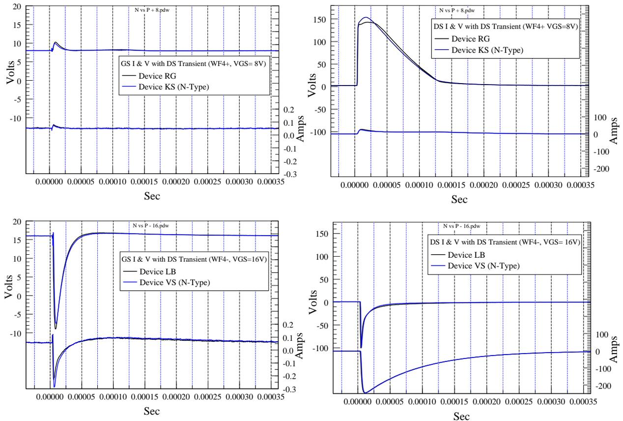
**Figure 18:** Comparison of Fail Levels with WF4+ and WF4- injected into MOSFET DS terminals. (WF4+, ③D-S pin config.  $V_{GS-bias} = 8$  Volts, Top: a & b.) (WF4-, ④ D-S pin config.  $V_{GS-bias} = 16$  Volts, Bottom: c & d.) for these data. The plots on the right (b & d) are the DS voltages and currents. The plots on the left (a & c) are the corresponding G-S voltages and currents resulting from the injection on the D-S terminals.
