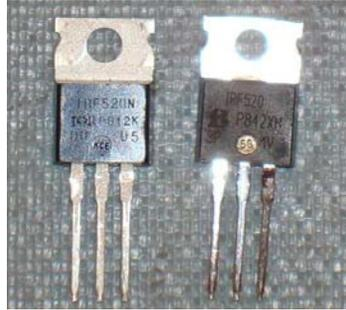
**Figure 17:** IRF520N (left) versus IRF520 (right, “shiny”) MOSFETS.
