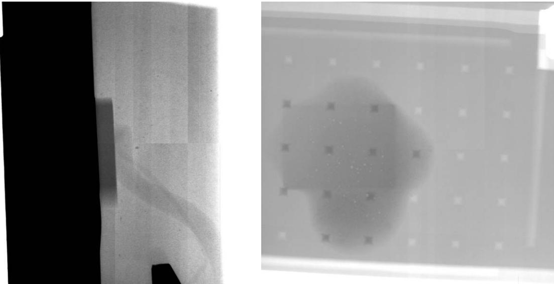
**Figure 22:** X-Ray images of IRF520N MOSFET die, adhesive and internal wiring.
