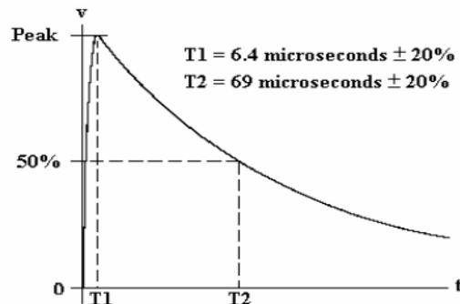
**Figure 2:** RTCA/DO-160E Section 22 Voltage Waveform 4.
