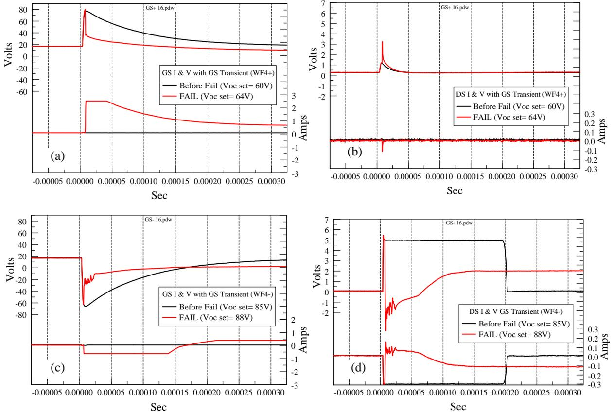
**Figure 15:** Comparison of Fail Levels with WF4+ and WF4- injected into MOSFET GS terminals. (WF4+,  $\odot$ -S pin config. Top: a & b) (WF4-,  $\ominus$ -S pin config. Bottom: c & d)  $V_{GS-bias} = 16$  Volts for these data. The plots on the left (a & c) are GS voltages and currents. The plots on the right (b & d) are the corresponding DS voltages and currents resulting from the injection on the GS terminals.
