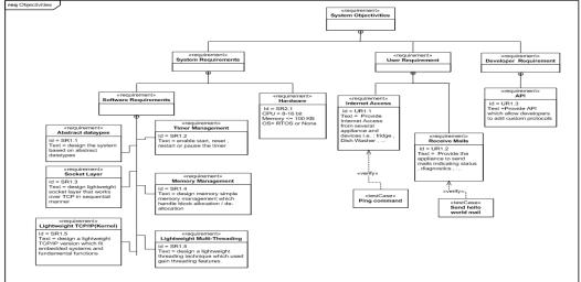
The proposed system requirement is classified into two categories both hardware and software
