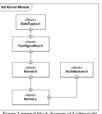
Figure 3 internal block diagram of Lightweight TCP/IP
