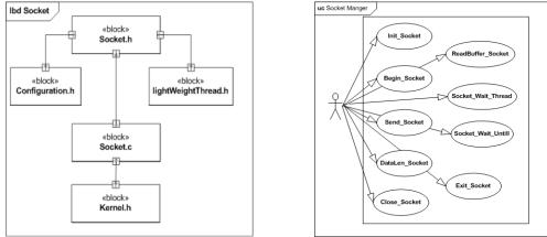
Figure 9 internal block diagram of socket manager
