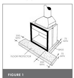
The floor protector must project a minimum of 300mm forward of the face of the Ligna unit and extend 200mm on each side of the unit. This must also be constructed of non-combustible materials at least 75mm thick as detailed above.
