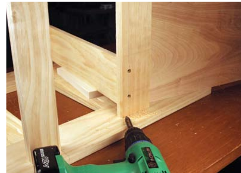
19 The slats were then screwed in place through the back stretcher of the chair. I used another scrap piece to hold the side slats \frac{3}{4} " off the side frame, then evenly spaced the other two slats between them. I used an 18-gauge pneumatic pin nailer to attach the front of the slats to the front stretcher. You could also use countersunk screws, or brad nails for this step.
