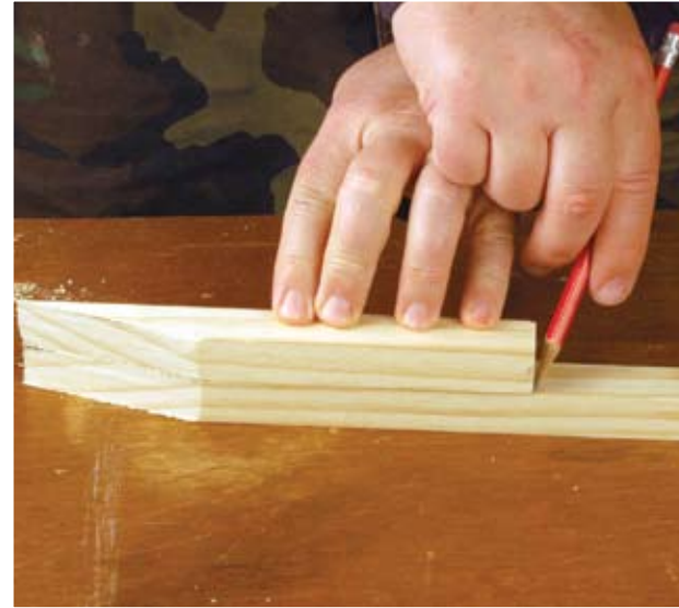
16 I then marked both pieces for length, and made the cuts.
