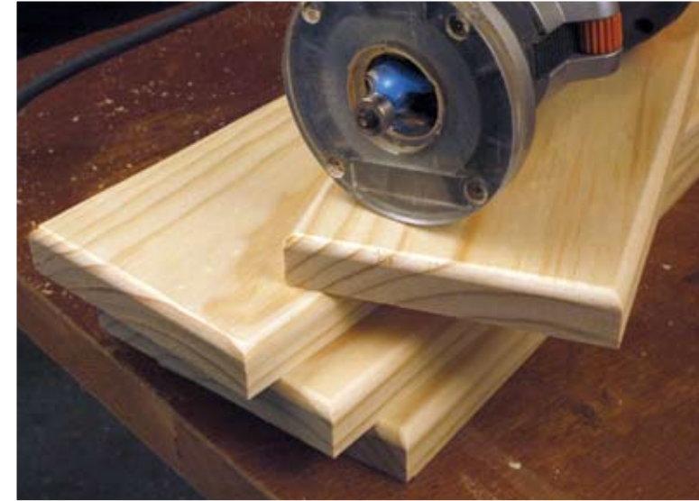
18 I then cut the seat slats to length and used my router to round over two long and one short edge on the top of the slats.
