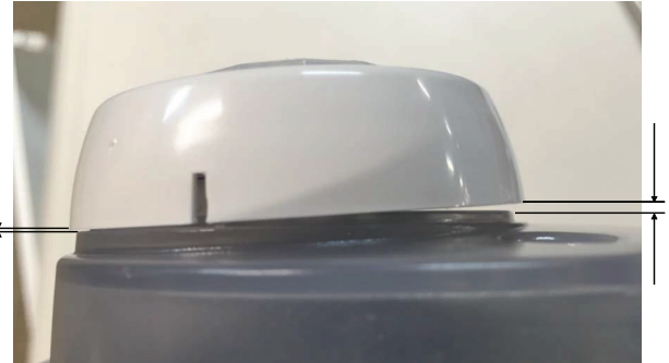
Uneven spacing around the perimeter
