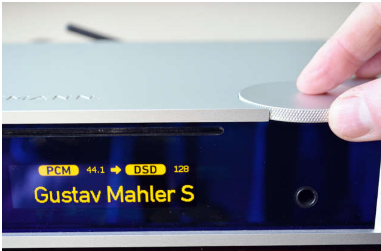
The Musicbook: 15 DSD can also be operated directly on the device. With the multifunctional wheel (which is also a volume control) you can reach all important points by means of a combination of pressing and turning. Here you can also see what the musicbook: 15 DSD commonly makes from the data of the CD: from PCM 44.1 becomes DSD 128
