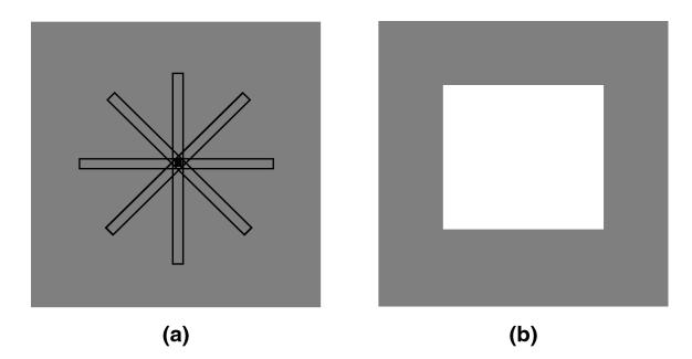
Figure 5: Conditions for a line. (a) The surrounding region has different graylevels from those of the pixels on the line. (b) The length is greater than its width.
