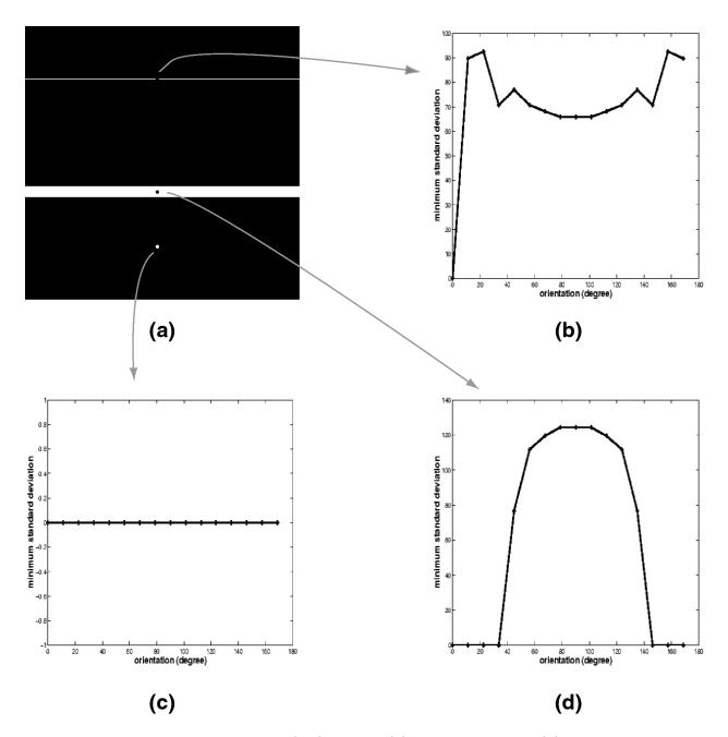
Figure 8: Relationship between  $\sigma_{i,j}(\theta, l)$  and  $\theta$ . (a) Original image. (b) Results for a pixel on the thin line. (c) Results for a pixel in the uniform region. (d) Results for a pixel on the thick line.
