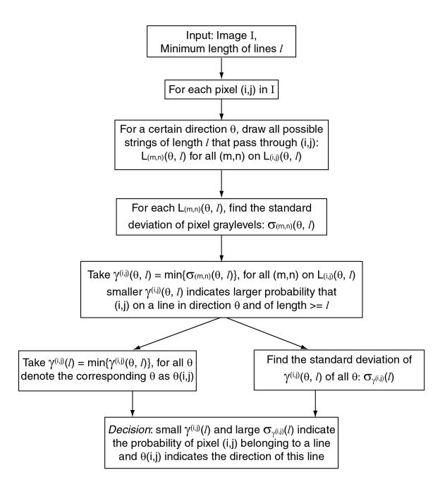
Figure 9: Block diagram of the line detector.
