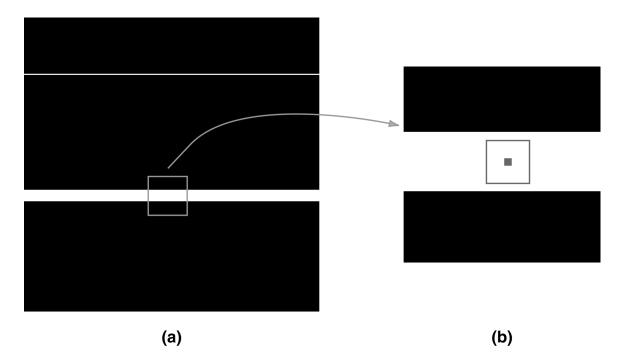
Figure 1: Pixels belonging to a line are not necessarily edge pixels. (a) An image with a 1 pixel wide "thin" white line at the top and a 10 pixel wide "thick" white line at the bottom. (b) The shaded pixel in the middle of the "thick" line looks unlike an edge pixel within a  $9 \times 9$  neighborhood.
