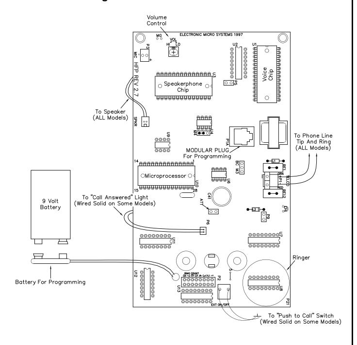
Note: On all HFP Rev. 2.7 or above revision boards, the jumper on P9 position should be installed whenever the phone is used with a cellular backup unit. When used on a regular phone line, the jumper should be removed.
