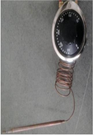
**Fig.12** Temperature sensor (thermostat)
