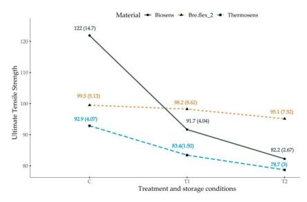
**Figure 4.** Treatment and storage conditions, and material as ultimate tensile strength predictors. Mean and standard deviation values in brackets () are presented for each group.
