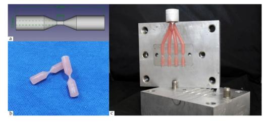
Figure 2. Test specimens' fabrication: (a) design; (b) finished test samples, (c) matrix form with injected specimens.
