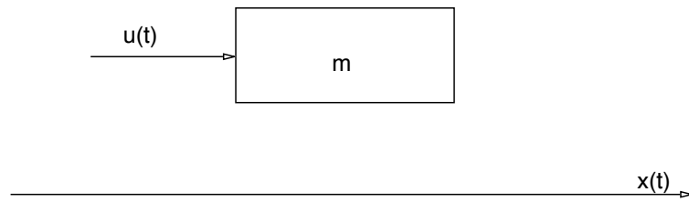
Figure 1.1: A body of mass m moving in one dimension under the influence of an external force u(t)
