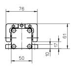
A1: depth 10 A2: funnel type lubricating nipple DIN3405-M6×1-D1 A3: socket cap screw ISO4762-M5×12 8.8
