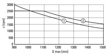
1: screw diameter 25 mm 2: screw diameter 32 mm
