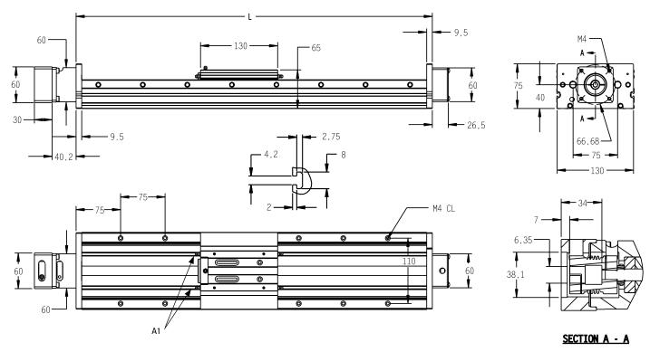
A1: lubrication nipples (using the unit with the nipples mounted makes the stroke 10 mm shorter).
