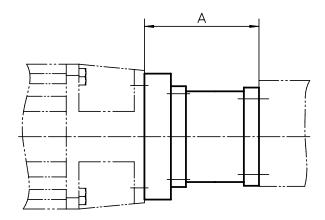
The bell house flange includes a matching coupling. Flanges for other units or motor sizes available on request, contact customer service. Note! Keep in mind that heavy motors will need extra support in order not to break the flange or gear due to the load torque created.
