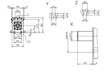
A1: depth 22 A2: socket cap screw ISO4762-M8×20 8.8
