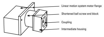
The standard NEMA motor mount sizes are listed above for reference. The Thomson RediMount™ System allows the linear units to be mounted to a wide variety of motor manufacturers and sizes. Many of these combinations can be found at www.linearmotioneering.com. Contact customer support for other motor sizes and their corresponding motor code.
