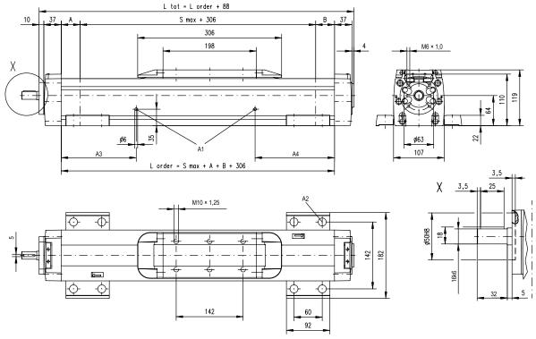
A1: lubrication holes A2: ø17/ø10,5 for socket head cap screw M10 A3: 100 (L order  $\leq$  1 m), 320 (L order > 1 m) A4: 100 (L order  $\leq$  1 m), 430 (L order > 1 m)
