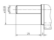
A1: depth 6 A2: lubricating nipple on both sides DIN3405 D 1/A
