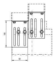
The limit switch brackets are adjustable in height. The limit switches on the brackets are operated by the maximum extended and maximum retracted end of stroke bars on top of the Z3 units. Two brackets are required.
