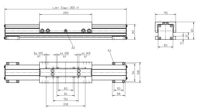
A2: funnel type lubricating nipple DIN3405-M6×1-D1
