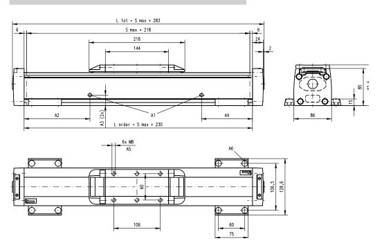
A1: lubrication holes ø6 (MG07N), ø10 (MF07N)
