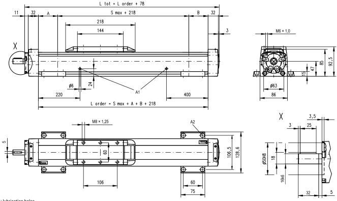
A1: lubrication holes A2: ø13,5/ø8,5 for socket head cap screw M8
