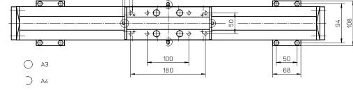
A1: depth 12 A2: socket cap screw ISO4762-M6×20 8.8
