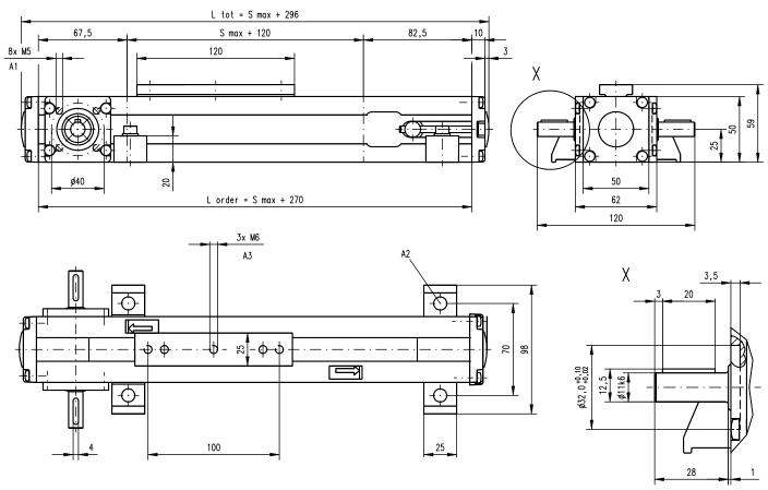
A1: depth 8,5 A2: ø6,5 for M6 screw A3: depth 9, Heli coil
