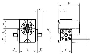
The worm gear is installed directly to the unit and requires no intermediate coupling between the two.
