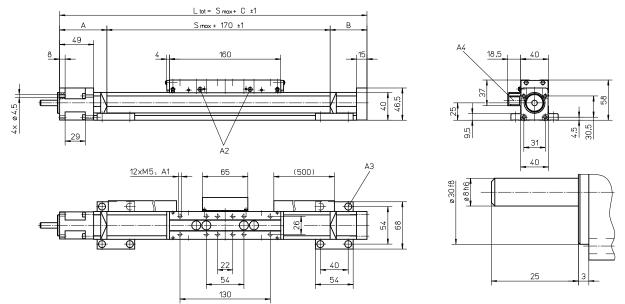
A1: depth 7 A2: lubricating nipple on both sides DIN3405 D 1/A A3: socket cap screw ISO4762-M5×12 8.8 A4: ENF inductive sensor rail kit (optional - see page 172)
