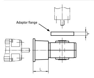
To be able to install the gear to the unit an adaptor flange must be used between the gear and the unit. The adaptor flange is ordered separately.
