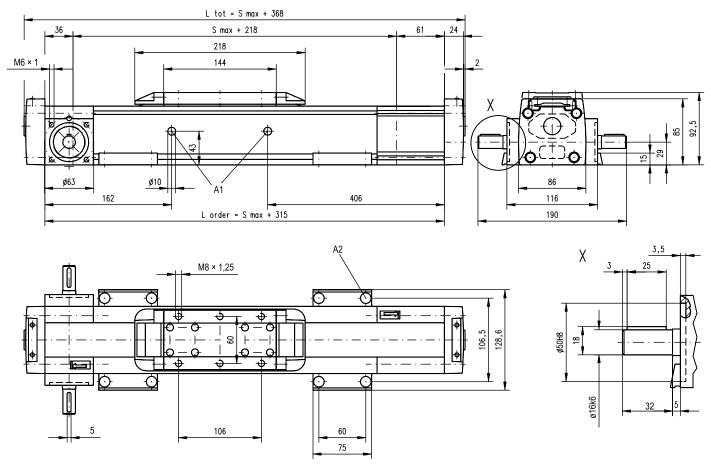
A1: lubrication holes A2: ø13,5/ø8,5 for socket head cap screw M8
