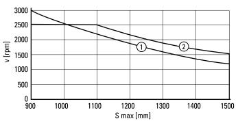
1: screw diameter 25 mm 2: screw diameter 32 mm
