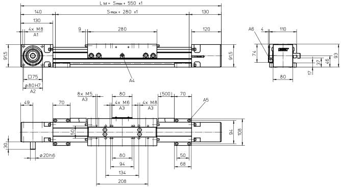
A1: depth 16 A2: depth 2,5 A3: depth 12 A4: funnel type lubricating nipple DIN3405-M6×1-D1 A5: socket cap screw ISO4762-M6×20 8.8 A6: ENF inductive sensor rail kit (optional - see page 172)
