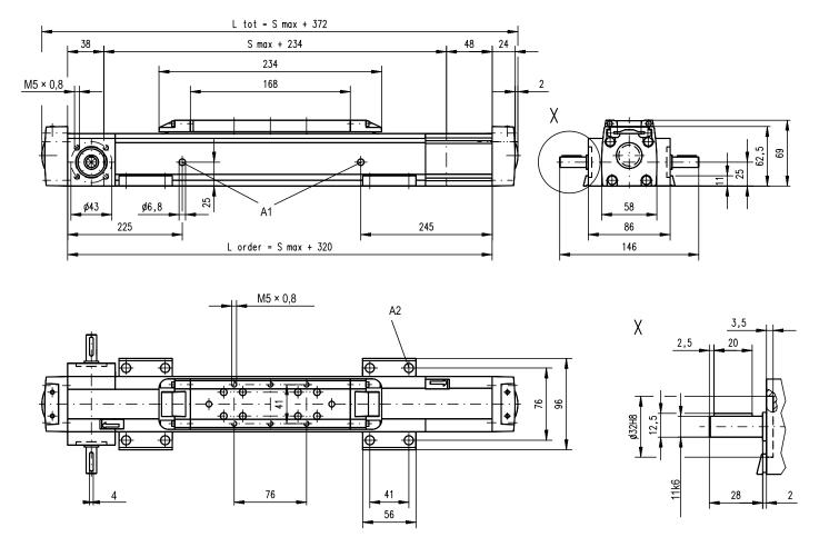
A1: lubrication holes A2: ø9,5/ø5,5 for socket head cap screw M5
