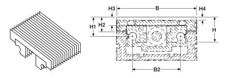
Bellows protect the unit from dirt and dust. Note that the bellows option reduces the available stroke of the unit by 28%. Bellows can be ordered and mounted at the factory - see ordering key. Bellows can also be ordered separately and fitted by the customer. In that case, order two pieces of bellows where the length of each bellows piece = stroke length of the unit  $\times$  0.86.
