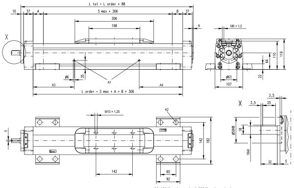
A1: lubrication holes A2: ø17/ø10,5 for socket head cap screw M10 A3: 100 (L order <= 1 m), 320 (L order > 1 m) A4: 100 (L order <= 1 m), 430 (L order > 1 m)
