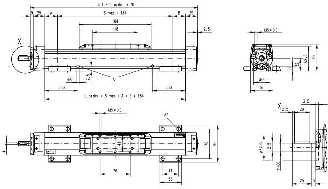
A1: lubrication holes A2: ø9,5/ø5,5 for socket head cap screw M5
