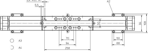
A1: depth 12 A2: socket cap screw ISO4762-M6×20 8.8 A3: tapered lubricating nipple to DIN71412 AM6
