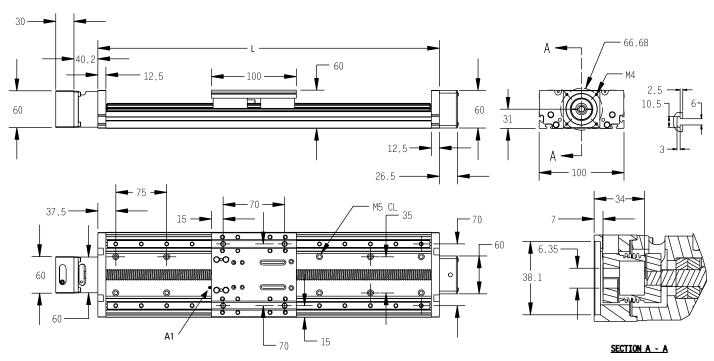
A1: lubrication nipple (using the unit with the nipple mounted makes the stroke 10 mm shorter).
