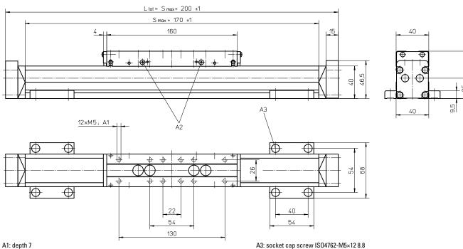
A1: depth 7 A2: lubricating nipple on both sides DIN3405 D 1/A
