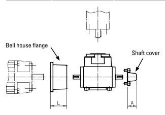
To be able to install the gear to the motor a bell house flange must be used between the gear and the motor. The bell house flange, which includes a matching coupling, is ordered separately. A shaft cover can be ordered to cover the second primary shaft on the gear in case it is not being used.
