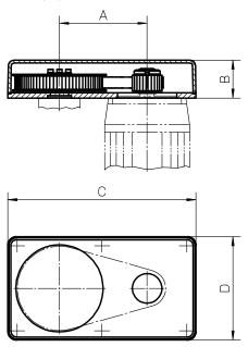
The belt gear comes in parts and is assembled to the unit and motor by the customer.
