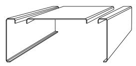
The protective shrouds are made of metal and protect the drive mechanism of the unit from dust and dirt but leave the guides unprotected. Shrouds do not reduce the stroke of the unit but they will add 4 mm to the width of the unit. Shrouds are ordered mounted from factory and are stated in the ordering key of the unit.
