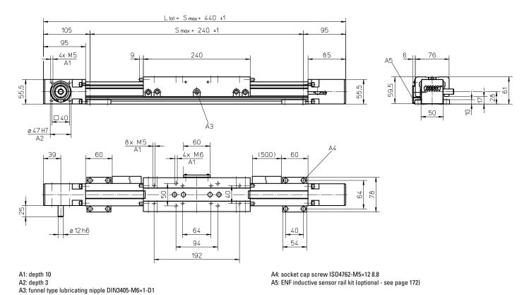
Long CarriageParameterWH50Carriage length[mm]400Dynamic load torque (My), maximum[Nm]130Dynamic load torque (Mz), maximum[Nm]75Weight[kg]1,47
