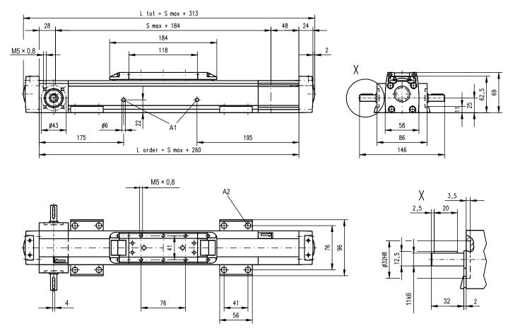
A1: lubrication holes A2: ø9,5/ø5,5 for socket head cap screw M5
