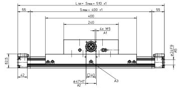
A1: depth 12 A2: depth 3,5 A3: funnel type lubricating nipple DIN3405-M6×1-D1 A5: depth 4
