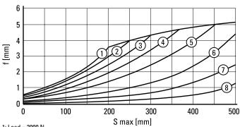
1: Load = 3000 N 2: Load = 2500 N 3: Load = 2000 N 4: Load = 1500 N 5: Load = 1000 N 6: Load = 500 N 7: Load = 250 N 8: Load = 125 N
