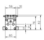
A1: depth 11 A2: socket cap screw ISO4762-M6×20 8.8 A3: tapered lubricating nipple to DIN71412 AM6
