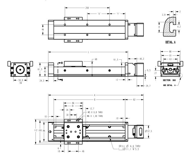
Standard NEMA23 motor dimensions are shown. Other mounting sizes are available and easily configured. Please see www.linearmotioneering.com for details.
