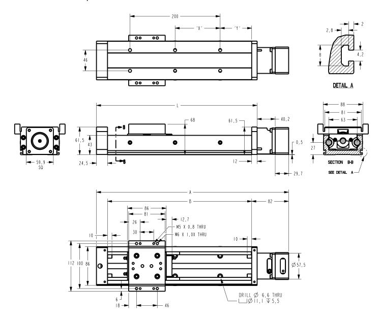
Standard NEMA23 motor dimensions are shown. Other mounting sizes are available and easily configured. Please see www.linearmotioneering.com for details.
