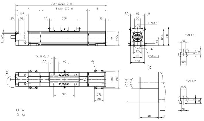
A1: depth 22 A2: socket cap screw ISO4762-M8×20 8.8
