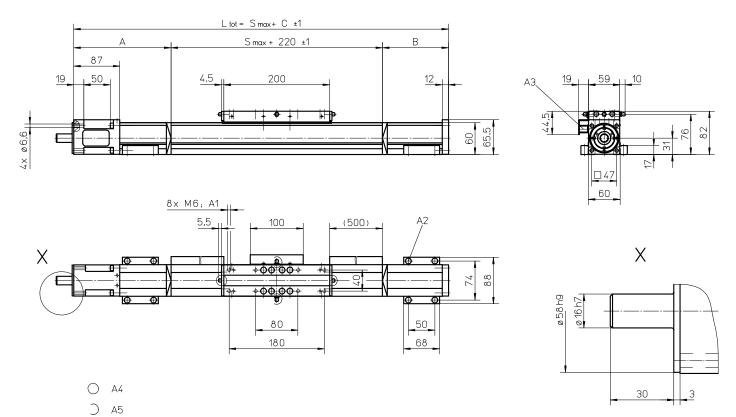
A1: depth 11 A2: socket cap screw ISO4762-M6×20 8.8
