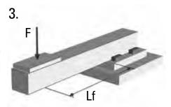
Profile supported in one end. Profile fixed at one side.
