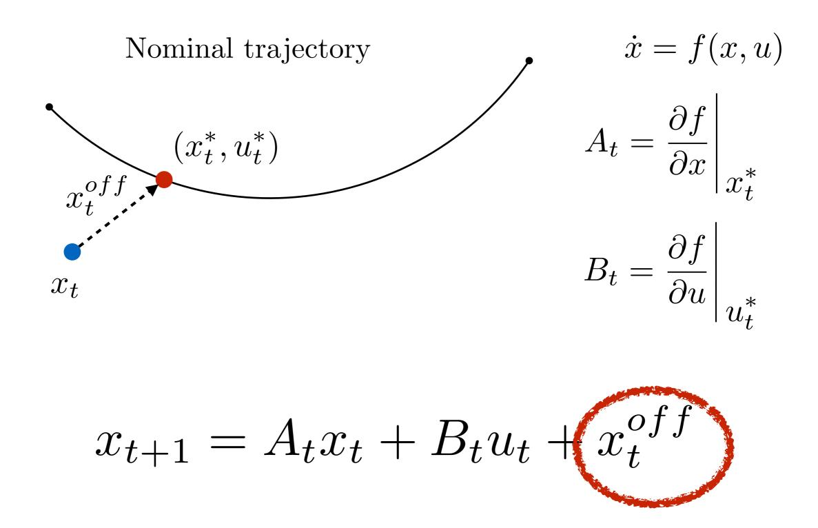
Trick to write in Linear System Form  $x_{t+1} = A_t x_t + B_t u_t + x_t^{off}$ Homogeneous coordinates  $\tilde{x} = \begin{pmatrix} x \\ 1 \end{pmatrix}$  $\tilde{x}_{t+1} = \begin{pmatrix} A_t & x_t^{off} \\ 0 & 1 \end{pmatrix} x_t + \begin{pmatrix} B_t \\ 0 \end{pmatrix} u_t$
