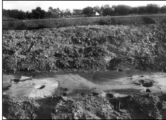
Figure 3. Photograph of sand boils along Coyote Creek in 1906 (Lawson, 1908).
