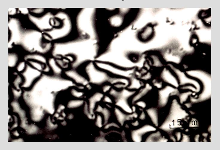
LC are birefringent and this micrograph shows typical disclination singularities that strongly influence the overall orientation of the whole sample
