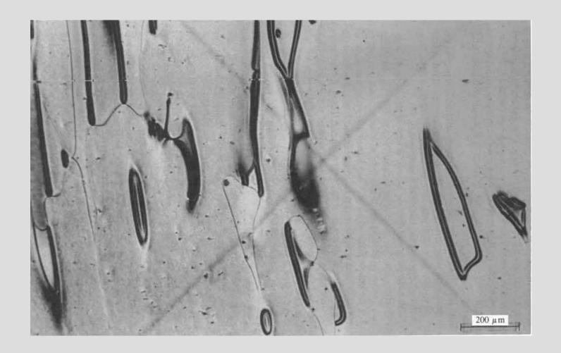
Disclination loops are common features in both LC and LCPs
