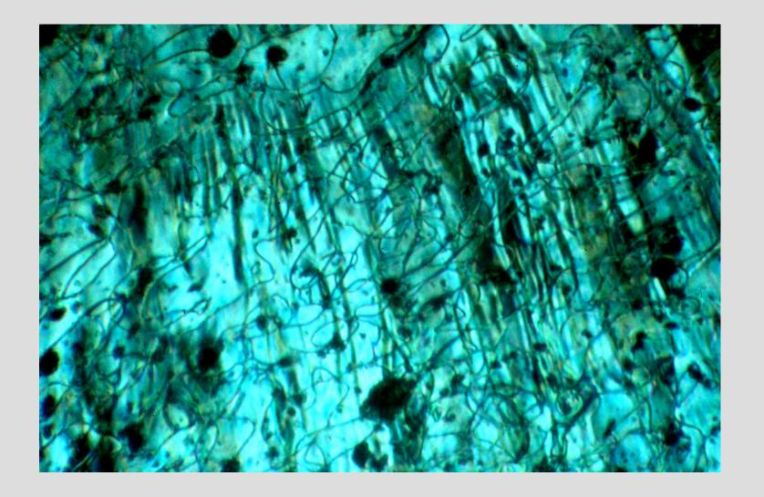
This micrograph shows a multitude of disclination loops within a thermotropic LCP melt
