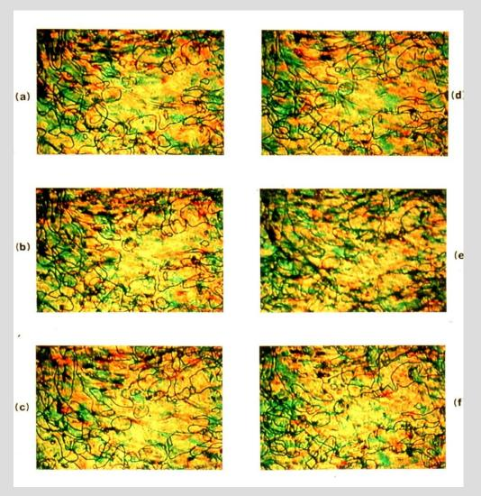
These micrographs show dense defect textures in LCPs and indicate that local orientational ordering of the LCP is controlled by the defect textue
