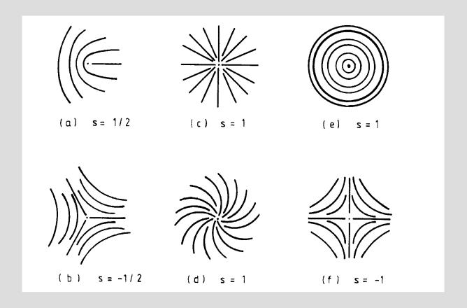
Liquid crystals invariably contain line defects known as "disclinations" and these disclinations have certain similarities to the more familiar "dislocations" that occur in metals and other crystals. F.C.Frank classified the type of disclinations that can occur in LCs and the diagram above shows the director orientation around different types of disclination singularities.
