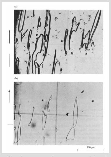
Disclination loops can be generated by shearing.
