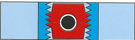
Load pin is free: Applied load conforms with set load. Blocking plate can be removed
