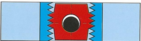
Load pin forced downwards: Applied load is higher than set load. Loosen connecting rod or increase set load
