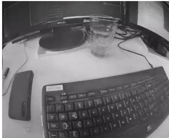
Reconstructed image from events (Samsung DVS)
