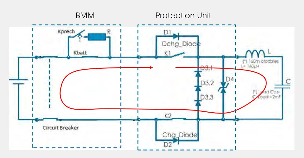
Discharge through diode with K1 open , but charge is stopped
