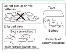
overheating, or explosion, so make sure to cover the (+) and (-) terminals with friction tape or some other insulator before disposal.
