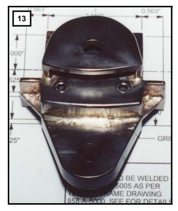
of the two Side Plates and Rear Plate as dimensioned in the drawing on page 6. They are then band saw cut to rough shape leaving as little material as possible to file, grind and/or mill to the finished dimensions.
