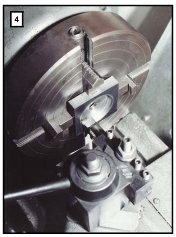
the two front corners which will be milled to their final shape in step 5, but first we need to make a clamping fixture in step 4.
