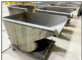
VIEW OF DUMPING HOPPERS
