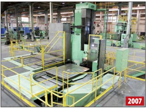
NOMURA BN-135QF CNC 4-AXIS FLOOR TYPE HORIZONTAL BORING MILL
