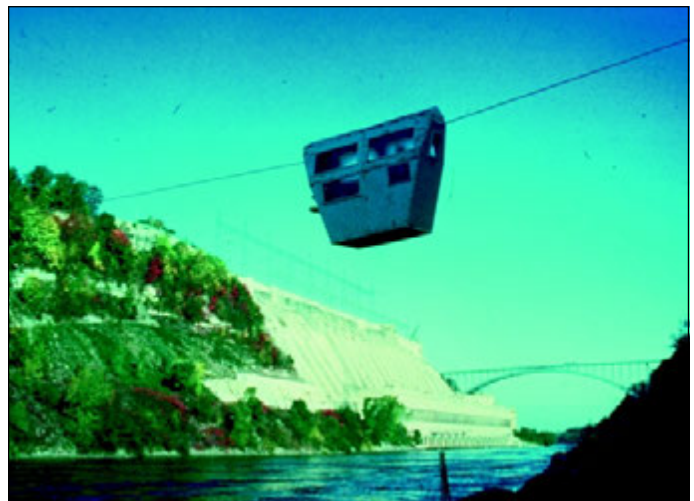
Measuring outflows at the Niagara Cableway across the Niagara Gorge
