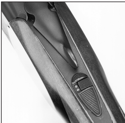
The safety incorporates the barrel selector; sliding it from left to right exposes two dots, indicating that the upper barrel will fire first. The Essential's trigger is an inertial type.
