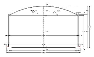
Figure 1 - Typical LNG tank cross-section
