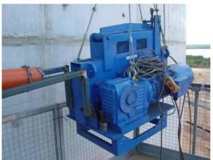
Figure 7 – High capacity strand pusher
