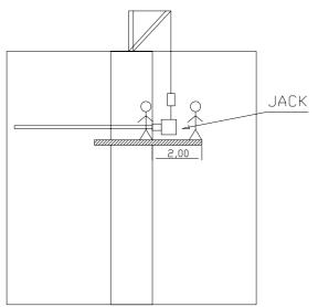
Figure 9 – Schematic showing handling of 2.5 tonne stressing jack.
