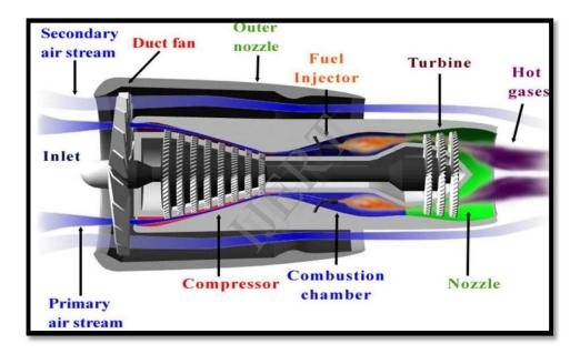
Fig 3: Turbofan Engines
