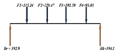
Total radial load acting on roller bearing  $Fr_{roller} = 3518.2 \text{ N} = 3.52 \text{ kN}$
