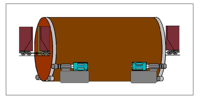
In all examples, the coupling between the motors is rigid and speed regulation is critical.
