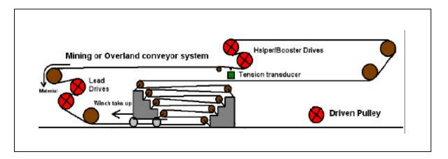
In these examples, the coupling between motors has a very high potential for oscillation; therefore, the automatic compensation inherent with the speed trim is best suited to these types of applications.
