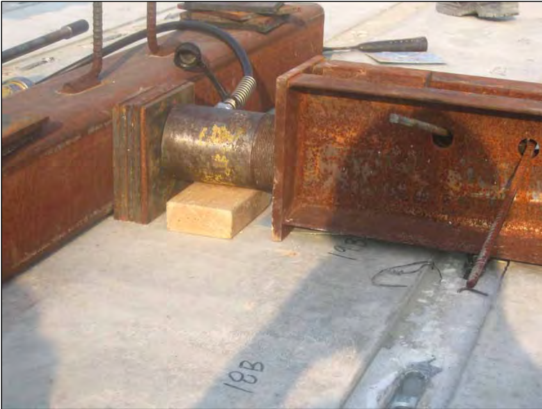
Figure A-16: Close-up photo of lateral shear test setup.
