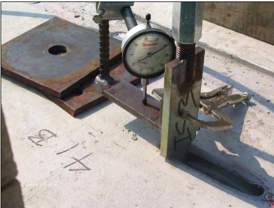
Figure A-13: Close-up photo of dial gage setup for pullout test.
