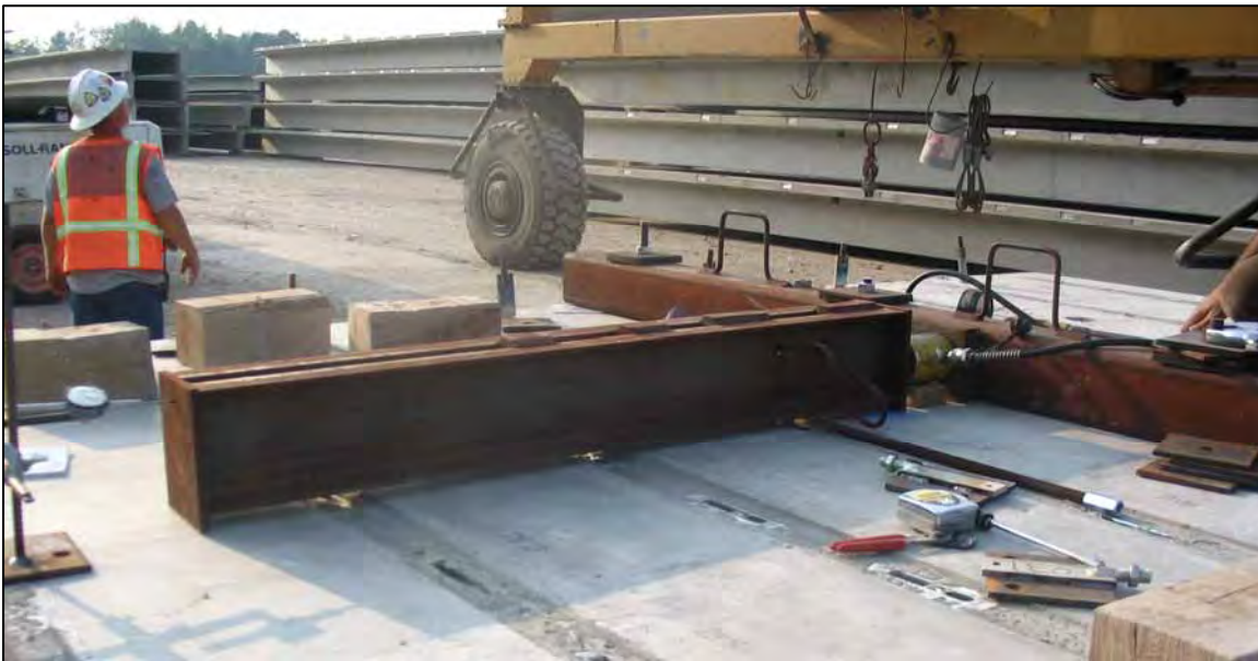
Figure A-15: Photo of lateral shear test setup.
