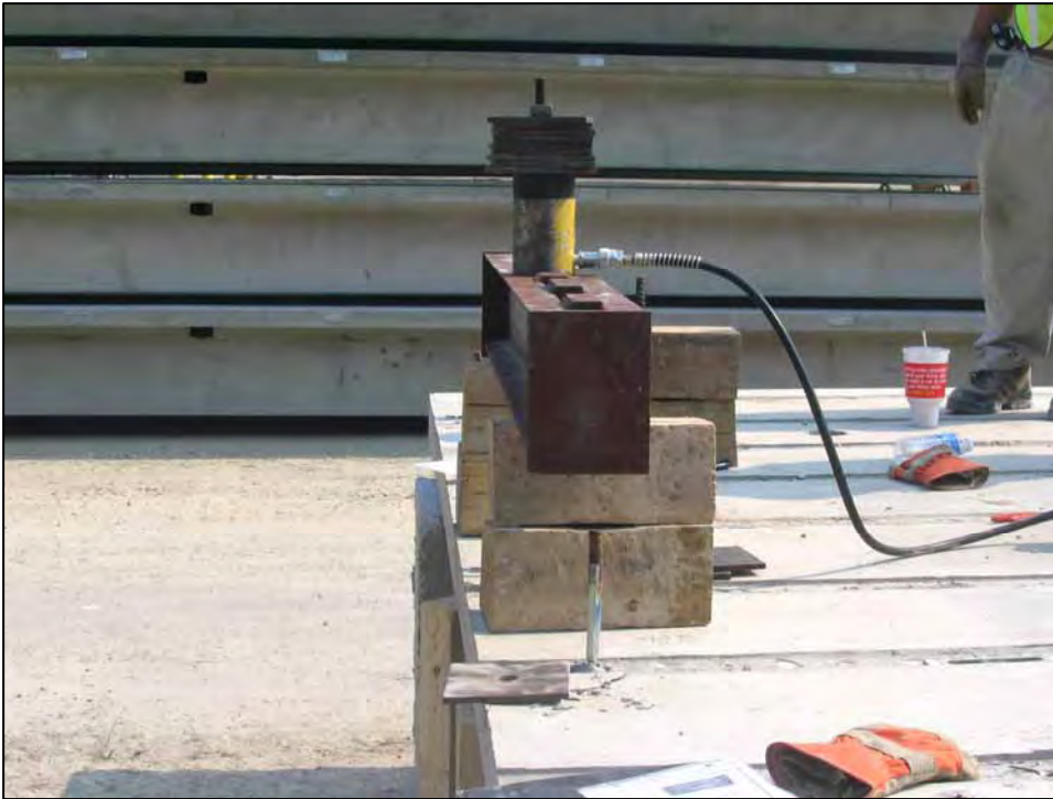
Figure A-12: Photo (side profile) of pullout test setup.
