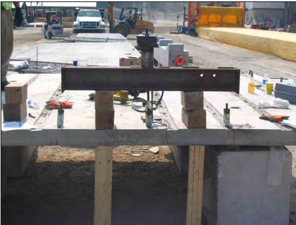
Figure A-11: Photo (front profile) of pullout test setup.
