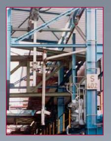
Built for chemical applications, the Emco Wheaton automatically operated Spot Loading System improves efficiency and accuracy without compromising on the highest hygiene and safety requirements. The unmanned operation results in low costs and reduction in human error.
