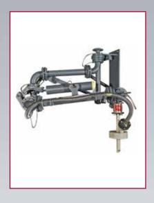
Specifically designed for the loading and unloading of acid and caustics such as 33% hydrochloric acid and 30% sulphuric acid, the Emco Wheaton loading arm for chemicals offers ease of use and safety features specifically tailored to applications with corrosive materials thanks to a protective PTFE lining.
