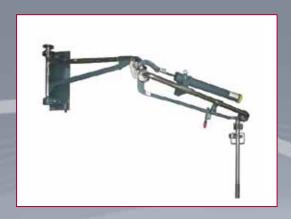
Specifically designed for the loading and unloading of small compartments such as drums or IBC containers, the Emco Wheaton Drum Filling Loading Arm avoids the disadvantages presented by traditional hose filling. The arm can be arrested in the working position to prevent slipping off the manhole and avoids the resulting waste of products and dangers associated with this.
