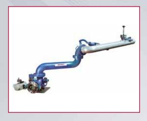
The Emco Wheaton E2704 with internal heating lance bottom loading arm is designed for petroleum applications with dense products that have been frozen or solidified. Hot product is pumped through the internal heating line and sprayed over frozen product, thawing it to be distributed via the product line of the loading arm.
