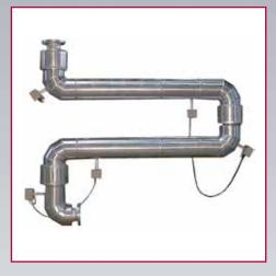
The Emco Wheaton Jumper Arm bridges variable distances between fixed connections. The two pipes are connected by a central axis which can twist to adapt to different distances between connections.
