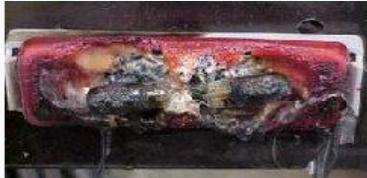
Compressed into foam seal, lights can reach 900 degrees F in as little as 20–30 minutes.
