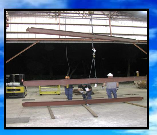
**Using our Rigging** Mock up s the Apprentice learns how to safely and skillfully apply slings, reeve blocks, use Chain falls, Come alongs, Snatch blocks, Tuggers and other various Rigging devices.
