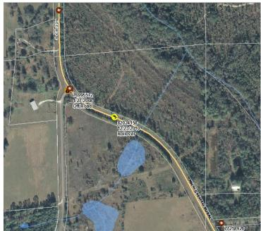
This typical base map shows road alignment, right of way, and water crossings.
